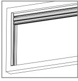
Insert the upper double rail between the two closing profiles.
