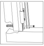
Drill and screw the profiles to the wall (screws not supplied).
