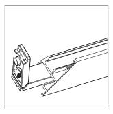
2 Insert the profile joint in the upper frame. Push it in the profile until you hear a click.
