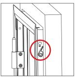
9 In case of irregularities adjust the adherence of the profile to the wall, with an Allen key.
