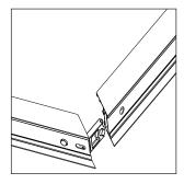
4 Insert the profile joint in the lateral profile forming the corner.
