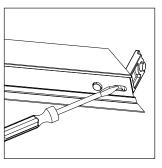
3 Loosen the screw of the profile joint.
