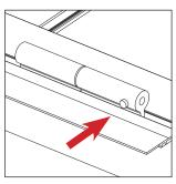
**13 FOR BACK HINGE VERSION ONLY:** adjust the spring tension using an Allen Key in the hinge, extracting the stop, screwing and unscrewing to adjust the tension, then insert the stop again in the hinge.
