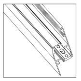
1 FOR TWO PANELS VERSION ONLY: insert the block bolt in the upper frame.
