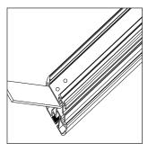
5 Insert the **short side** of the profile joint in the upper profile.
