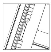
**2** Drill the lateral profiles for fixing the insect screen.
