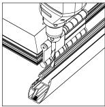
3 Drill two holes at the ends of the lateral profiles by calculating the width of the **long side** of the profile joint.
