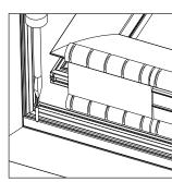
Drill and screw repeating the operation of inserting the profile joint on the opposite profile.
