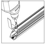
4 Drill two holes at the ends of the upper profile, by calculating the width of the **short side** of the profile joint.
