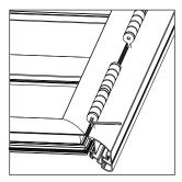
1 Loosen the spring tension and remove the locking pivot.
