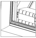
**10** Circle the holes to drill on the profile joint.
