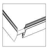
9 Insert the profile joint in the lateral profile.
