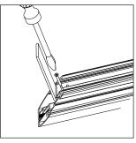
8 Screw the profile joint on the upper profile (screws not supplied).
