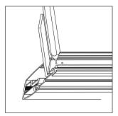
6 Circle the holes to drill on the profile joint.
