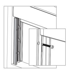
Place the latch-guide profile and fix it with the proper screws in the arranged holes.
