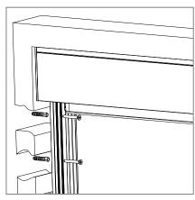
**3** Fix the side guides using the proper holes.
