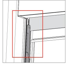
▲ Insert the inner guide and ensure that the zip enter the plastic scroll profile.
