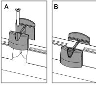
Repeat the step nr. 9 with the other lower rail and insert the central joint. Fix it in the floor (A) and insert the cap for the screw (B).
