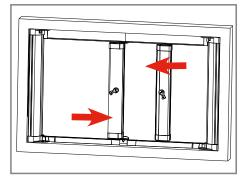
**11** Carefully verify the proper winding to make sure that the conveyors are properly inserted in their sliders.
