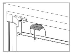
Adjust any irregularities of the window tightening the screw in the upper compensating profile.
