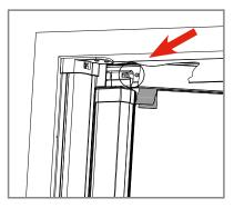
7 Insert the upper rails using the paper tab to get the conveyor of the mesh in the cylindrical space of the slider.
