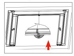
8 Insert the upper rails in the caps of the cassette and join them in the middle with the central joint.
