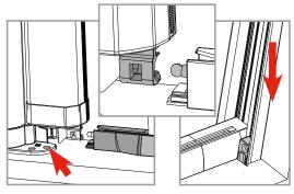
Insert the bottom guide in the latch-guide of the box: with the help of the paper tab, be sure that the latch for mesh enters the cylindrical seat of the slider. Insert the closure profile. Insert the opposite side of the bottom guide in the closure profile and block it with the appropriate latch-guide.
