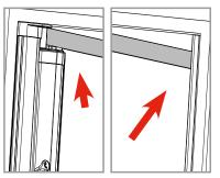
**9** Insert the compensating profile in the box first, then in the closure profile.
