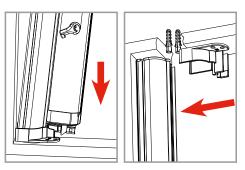
2 Hook the box to the head-cap. Hook the other head-cap to the box and apply into the window recess.
