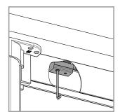
Screw the grub screws on the upper compensating profile to adjust the possible irregularities of the wall.
