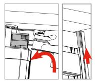
12 Insert the top guide in the latch-guide of the box: with the help of the paper tab, be sure that the latch for mesh enters the cylindrical seat of the slider.
