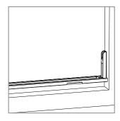
Apply the lower rail complete with bayonet mounts to the floor, using the double-sided tape.
