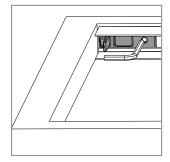
When the bayonet mount is secured to the wall, lock it into the upper rail by tightening the relevant grub screw.
