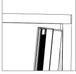
Insert the back bar and handle bar, left and right, into the top rail and then move them towards the wall.
