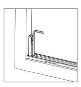
Ensure the bayonet mount adheres perfectly against the wall and then lock it into the lower rail, tightening the relevant grub screw.
