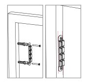
Secure the lateral profiles to the walls in order to trace their exact location on the wall, marking this with a pencil. Apply the fixing clips (the use of clips when the height exceeds 160 cm is recommended).
