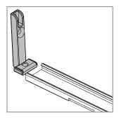
Insert the bayonet mounts into the lower rail on both sides, ensuring they adhere perfectly to the wall.
