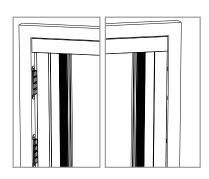
Apply the lateral profile with the handle bar, pressing on the fixing clips.
