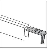
1 Insert the bayonet mounts on the top rail from both sides as shown in the photos so that the latter adheres perfectly against the wall.
