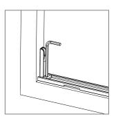
6 Ensure the bayonet mount adheres perfectly against the wall and then lock it into the lower rail, tightening the relevant grub screw.
