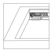
When the bayonet mount is secured to the wall, lock it into the upper rail by tightening the relevant grub screw.
