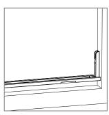
Apply the lower rail complete with bayonet mounts to the floor, using the double-sided tape.
