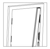
8 Insert the corresponding profile below the lower guide securing it to the side wall, gently sliding along the lower rail press on the locking clips.
