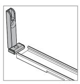
4 Insert the bayonet mounts into the lower rail on both sides, ensuring they adhere perfectly to the wall.
