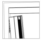
9 Insert the back and handle bar into the top rail and then move them towards the wall.
