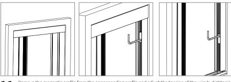
Remove the magnetic profile from the corresponding profile and adjust the tension of the wire by tightening the two grub screws located inside. CAUTION! Do not tighten the cords up too much, because they could break when using the flyscreen.
