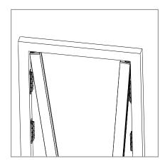
Insert the corresponding profile below the lower guide securing it to the side wall, gently sliding along the lower rail press on the locking clips.
