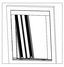
9 Insert the back and handle bar into the top rail and then move them towards the wall.
