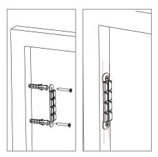
Secure the lateral profiles to the walls in order to trace their exact location on the wall, marking this with a pencil. Apply the fixing clips (the use of clips when the height exceeds 160 cm is recommended).
