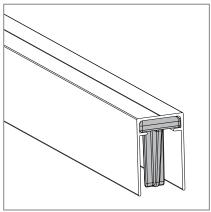
Insert the bayonet mounts on the top rail from both sides as shown in the photos so that the latter adheres perfectly against the wall.
