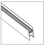
6 Remove the magnetic sheath from the back profile.
