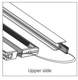
7 Insert the pull cord in the upper side of the back profile.
