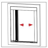
6 Make sure that the closure profile and the handlebar are fixed to the frame.
