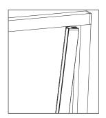
4 Insert the handlebar under the upper rail adhering it to the frame.
