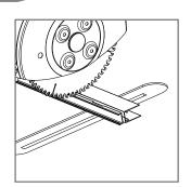
2 Cut the lower and upper guide according to the desired sizes, subtracting 2 mm.
