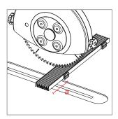
Starting from the finished mesures of the insect screen, cut the mesh by subtracting another 24 mm.
