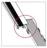
2 Insert the mesh in the handlebar.
