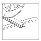
4 Cut the side guide according to the desired sizes, **subtracting 30 mm**.
