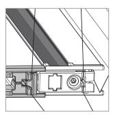
Fix the wires in the slots provided on the plugs.
