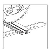
Cut the handle bar according to the desired sizes, **subtracting** 33 mm.
