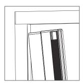
Insert the closure profile under the upper rail and adhere it to the frame.
