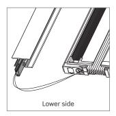
Insert the pull cord in the lower side of the back profile.
