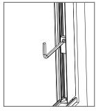
**5** Apply the insect screen and adjust the position of the pull cord.
