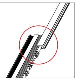
3 Insert the mesh in the back profile with no magnet.
