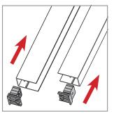
Insert the bottom corners in the side guides of the frame. Fix the corners with the screws.
