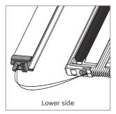
Insert the cut plug in the back profile; be sure to release the cord from the groove.
