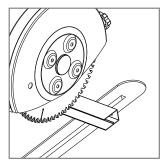
1 Cut the profiles for front attachment according to the desired sizes, **subtracting 44 mm**. (E.g. 1300 mm = cut 1256 mm).
