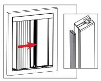
Verify the proper functioning of the insect screen and insert the magnetic sheathing into the back profile.
