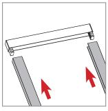
Assemble the frame coupling the side guides to the upper rail.
