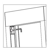
Fix the upper rail to the side guides using the screws.
