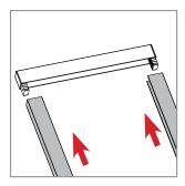
Assemble the frame coupling the side guides to the upper rail.
