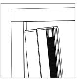
4 Insert the handlebar under the upper rail adhering it to the frame.
