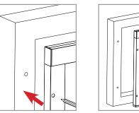
Fix the frame to the wall using the holes on the side guides. Use the caps by pushing them into the holes.
