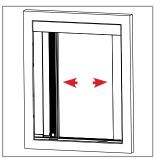
Make sure that the closure profile and the handlebar are fixed to the frame.
