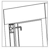
Fix the upper rail to the side guides using the screws.
